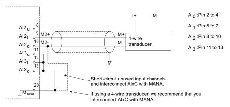
Figure 8-2 Connection of a 4-wire transducer to an analog current/voltage input of the CPU 313C/314C-2
