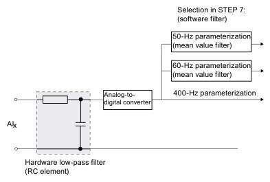
Figure 8-4 Principle of interference suppression with STEP 7
