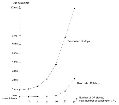
With multi-master operation on a PROFIBUS DP network, you must make allowances for the DP cycle time for each master. That is, you will have to calculate the times for each master separately and then add up the results.
