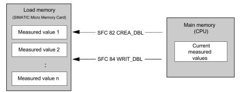
• You can call SFC 82 "CREA\_DBL" in the user program to generate new (additional) nonruntime-relevant DBs in load memory which do not require main memory space. 5.2 Memory functions
