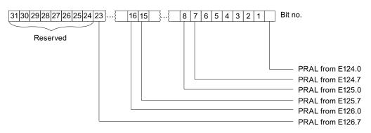
Figure 8-9 Displaying the statuses of CPU 31xC interrupt inputs
