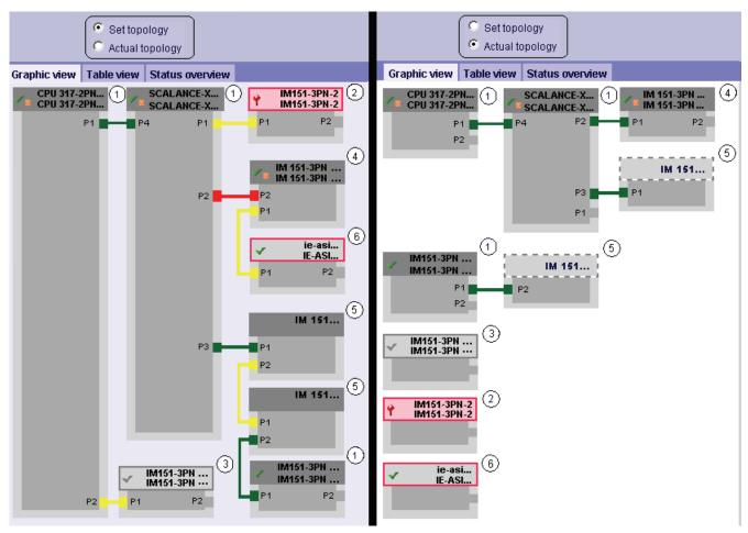
Figure 3-14 Graphical view - Target and actual topology
