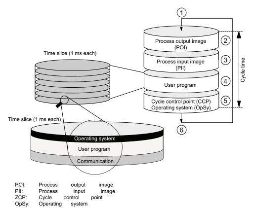
In contrast to S7-400 CPUs, the S7-300 CPUs data only allow data access with an OP/TP (operator control and monitoring functions) at the cycle control point (data consistency, see the technical specifications). Program execution is not interrupted by the operator control and monitoring functions.
