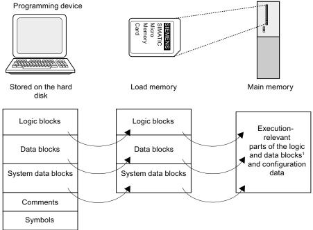
The figure shows the load and main memory of the CPU
