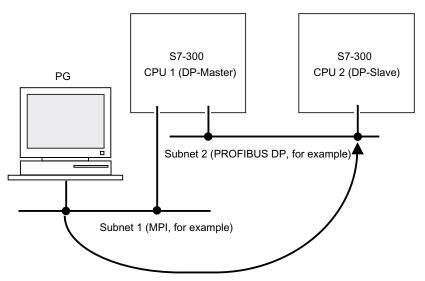
The figure below shows the MPI access to PROFINET via PROFIBUS. CPU 1 (e.g. 315-2 DP) is the gateway between subnet 1 and 2; CPU 2 is the gateway between subnet 2 and 3.
