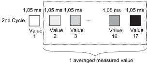
Figure 8-6 60 Hz interference frequency suppression
