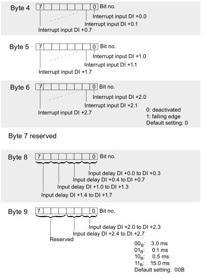
Figure 8-7 Structure of the data set 1 for standard DI and interrupt inputs (length of 10 bytes)
