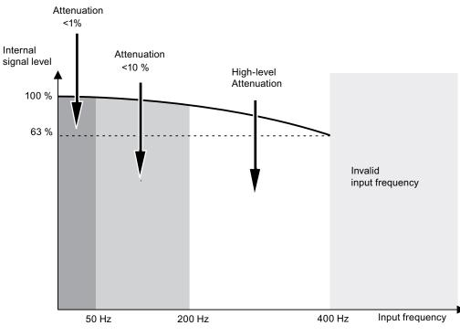
Figure 8-3 Low-pass characteristics of the integrated filter
