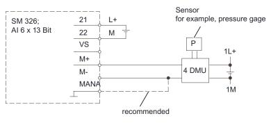
Figure 9-6 External encoder supply, 4-wire transducer for SM 336; AI 6 x 13Bit
