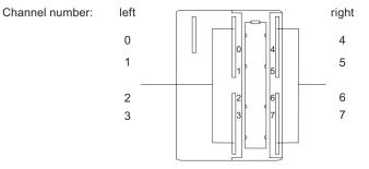
Figure 8-35 Channel numbers of SM 326; DO 8 x DC 24 V/2A PM
