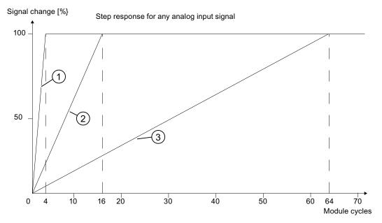
Figure 9-38 Example of effect of smoothing on step response
