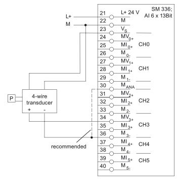
Figure 9-12 Voltage measurement 0 to 10 V for application 1 with SM 336; AI 6 x 13Bit
