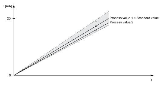
Figure 9-39 Example of a relative tolerance window *without* discrepancy (parameter assignment: standard value = MAX)
