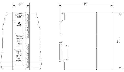
Figure B-4 Dimensions of the safety protector
