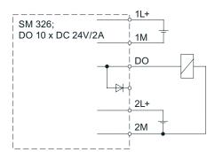
Figure 8-45 Wiring scheme of SM 326; DO 10 x DC 24V/2A for applications 1, 3 and 5
