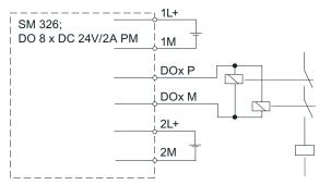
Figure 8-39 Wiring scheme of two relays on a digital output of SM 326; DO 8 x DC 24V /2A PM – Controlling cross circuits
