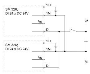
Figure 8-11 Wiring scheme of SM 326; DI 24 x DC 24V for application 4 with single-channel connection of one sensor
