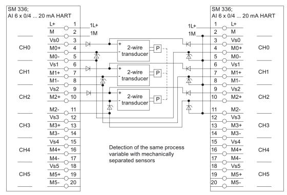
Figure 9-36 2003 evaluation, redundant F-SMs, transducer via 3-channels
