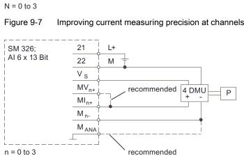
Improving current measuring precision at channels 0 through 3 using 2 DMU
