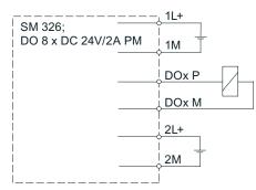
Figure 8-37 Wiring scheme of SM 326; DO 8 x DC 24V/2A PM for applications 1 and 2
