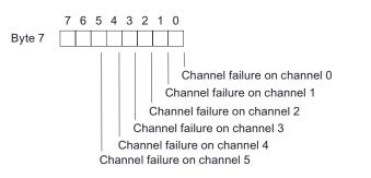
Figure A-8 Diagnostics data byte 7 for SM 326; AI 6 x 13 Bit
