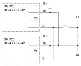
Figure 8-8 Wiring scheme of SM 326; DI 24 x DC 24V for application 2 with single-channel connection of one sensor
