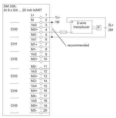
Figure 9-23 2-wire transducer, external sensor supply
