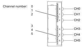
Figure 9-20 Channel numbers SM 336; F-AI 6 x 0/4 ... 20 mA HART
