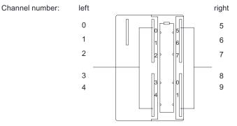
Figure 8-43 Channel numbers of SM 326; DO 10 x DC 24V/2A
