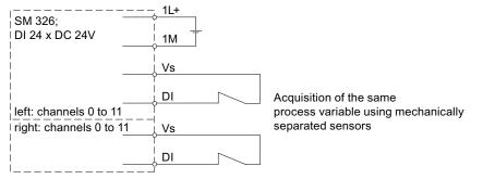
Figure 8-17 Wiring scheme of SM 326; DI 24 x DC 24V for application 5 with two-channel connection of two single-channel sensors
