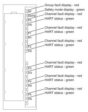
Figure 9-18 Front view SM336; F-AI 6 x 0/4 ... 20 mA HART
