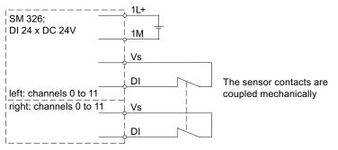
Figure 8-16 Wiring scheme of SM 326; DI 24 x DC 24V for application 5 with two-channel connection of one two-channel sensor
