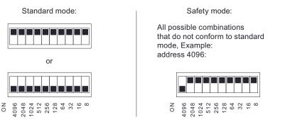
Figure 4-1 Example of address switch (DIP switch) settings
