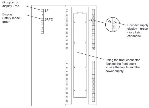
Figure 9-2 Front view of SM 336; AI 6 x 13Bit
