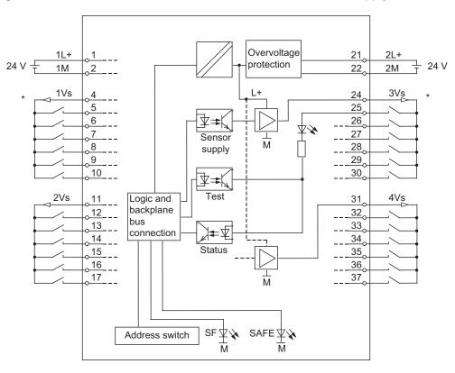
\* The representation of NO contacts matches the module labeling. Usually, the sensors must be equipped with NC contacts in order to ensure the safe state of process variables.
