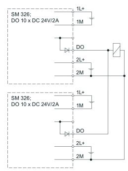
Figure 8-47 Wiring scheme of SM 326; DO 10 x DC 24V/2A for applications 2, 4, and 6
