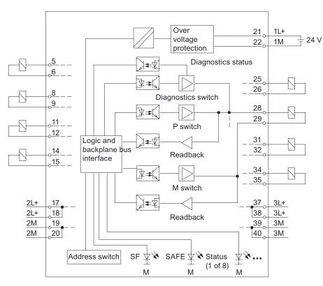
Figure 8-34 Wiring and block diagram of SM 326; DO 8 x DC 24V/2A PM
