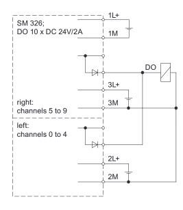
Figure 8-48 Wiring two outputs of SM 326; DO 10 x DC 24V/2A in parallel for dark period suppression
