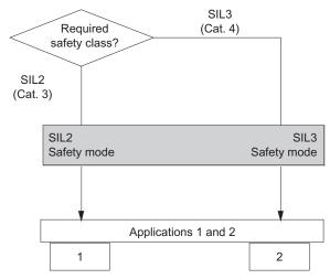
Figure 8-36 SM 326; DO 8 x DC 24V/2A PM - Selecting an application
