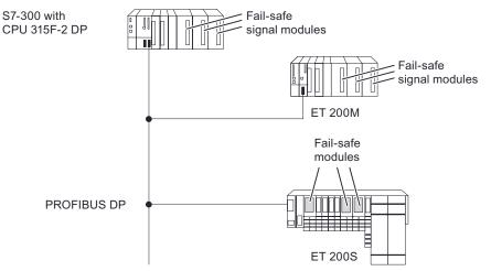
Figure 1-1 Fail-safe S7 Distributed Safety automation system
