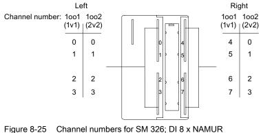
1002 evaluation of the sensors reduces the number of channels by half.
