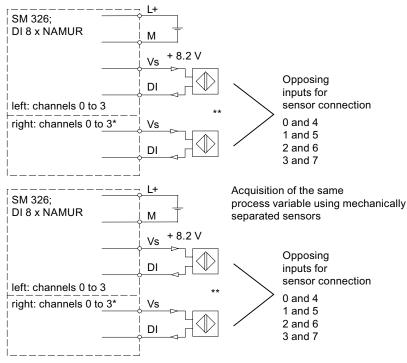
\*The left channels return the user signals \*\* optional mechanical coupling of sensor contacts
