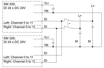
\* Sensor contacts are mechanically coupled; alternatively, you can connect two single-channel sensors
