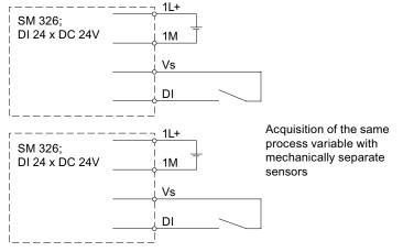
Figure 8-9 Wiring scheme of SM 326; DI 24 x DC 24V for application 2 with single-channel connection of two redundant sensors
