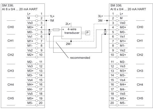
Figure 9-29 4-wire transducer, external sensor supply with module redundancy
