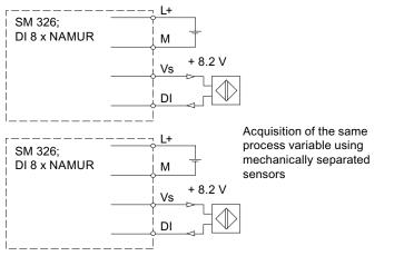
Figure 8-29 Wiring scheme of SM 326; DI 8 x NAMUR for applications 2 and 4
