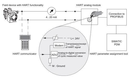
Figure 9-45 System environment for HART applications
