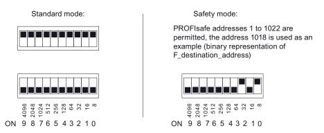
Figure 4-2 Example of address switch (DIP switch) settings
