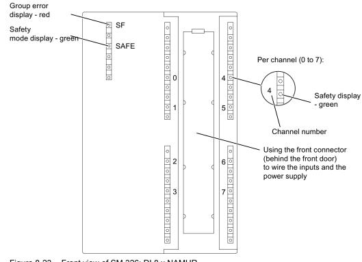
Figure 8-23 Front view of SM 326; DI 8 x NAMUR
