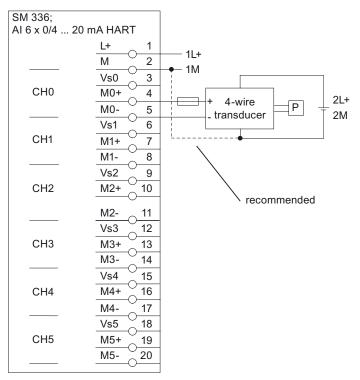
Figure 9-25 4-wire transducer, external sensor supply
