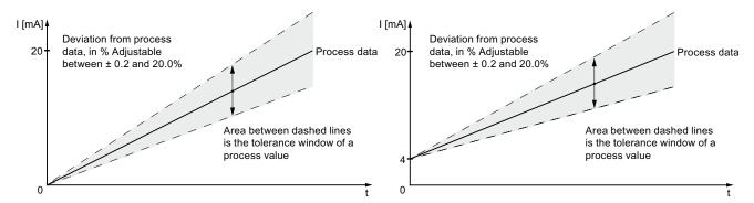
Figure 9-42 Relative deviation in % of the nominal range for measuring range 0 to 20 mA or 4 to 20 mA
