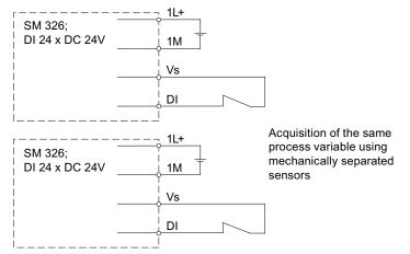
Figure 8-12 Wiring scheme of SM 326; DI 24 x DC 24V for application 4 with single-channel connection of two redundant sensors
