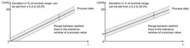
Figure 9-41 Absolute deviation in % of the nominal range for measuring range 0 to 20 mA or 4 to 20 mA
