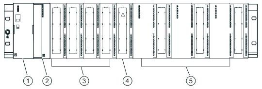
Figure 10-3 Configuration of ET 200M with safety protector (hot-swapping of the module not supported)
