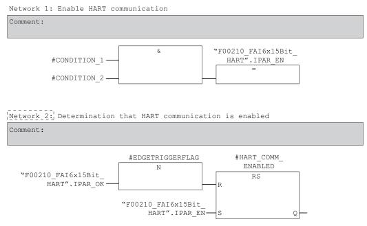
Figure 9-47 Example of enabling HART communication in S7 Distributed Safety
