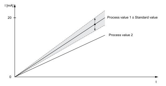
If the process value does not represent the standard value at an instant but is outside the tolerance window, a discrepancy exists.
