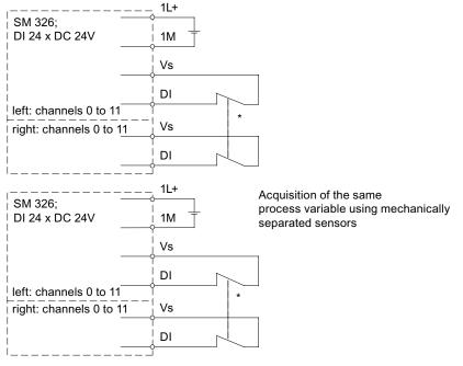
\* Mechanically coupled sensors; alternative connection of two single-channels sensors
