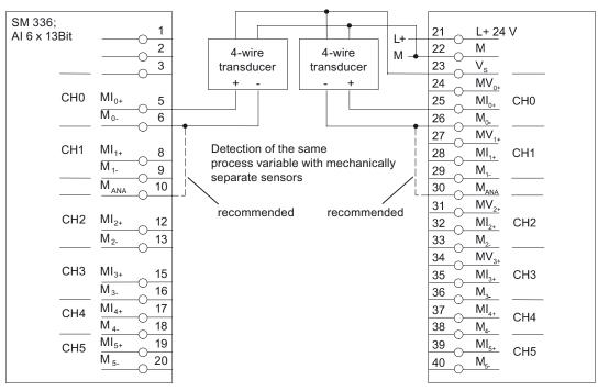
Figure 9-16 Current measurement 4 to 20 mA, 4-wire transducer for application 5 with SM 336; AI 6 x 13Bit
