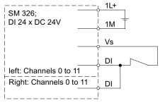
Figure 8-13 Wiring scheme of SM 326; DI 24 x DC 24V for application 5 with single-channel connection of one sensor
