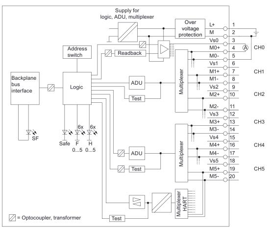
Figure 9-19 Wiring and block diagram of SM 336; F-AI 6 x 0/4 ... 20 mA HART
