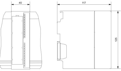
Figure B-2 Dimension drawing SM 336; F-AI 6 x 0/4 ... 20mA HART
