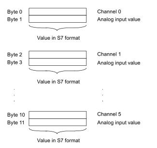
Figure 9-51 Input user data area of the HART analog modules
