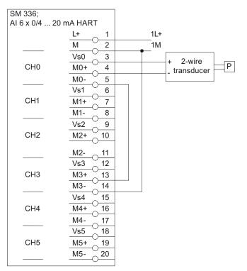
Figure 9-33 1002 evaluation, transducer via 1-channel
