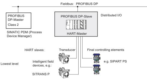
Figure 9-44 Location of use of the HART analog modules in the distributed system
