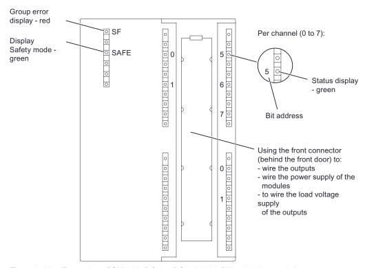
Figure 8-33 Front view of SM 326; DO 8 x DC 24V / 2A PM; with diagnostic interrupt
