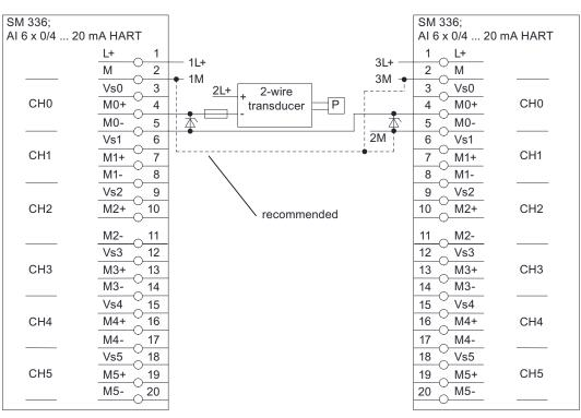
Figure 9-27 2-wire transducer, external sensor supply with module redundancy
