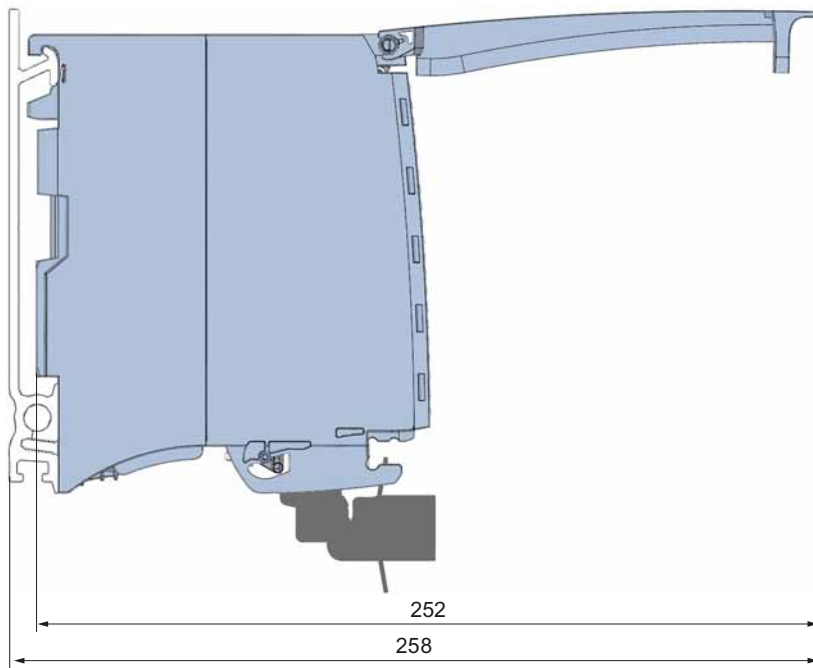
Figure A-2 Dimensional drawing of the AQ 4xU/I ST module, side view with open front panel
