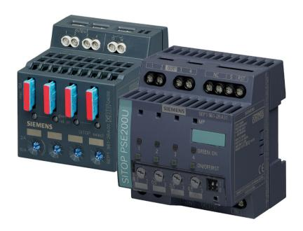
In conjunction with a 24 V power supply, the selectivity module is used to distribute the load current across several branches and to monitor the individual currents in these branches. Faults in the individual branches caused by overload or short-circuit are detected and selectively switched off, so that the fault does not impact the other load circuits. This means fast troubleshooting and minimized downtimes.
