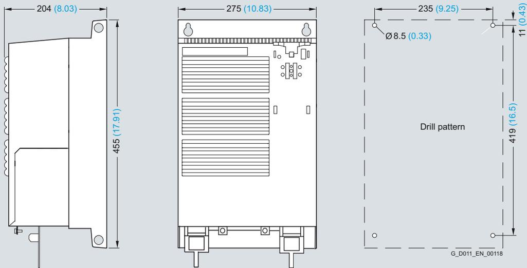
PM260 Power Module frame size FSD with and without integrated class A line filter
