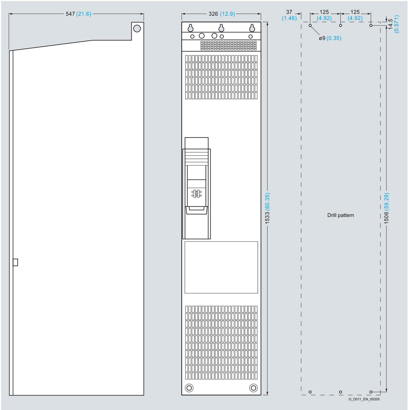
PM240 Power Module frame size FSGX without line filter
