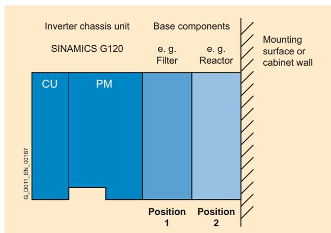
Frequency inverters comprising a Power Module (PM) and a Control Unit (CU) and two base components at position 1 and position 2 (side view)
