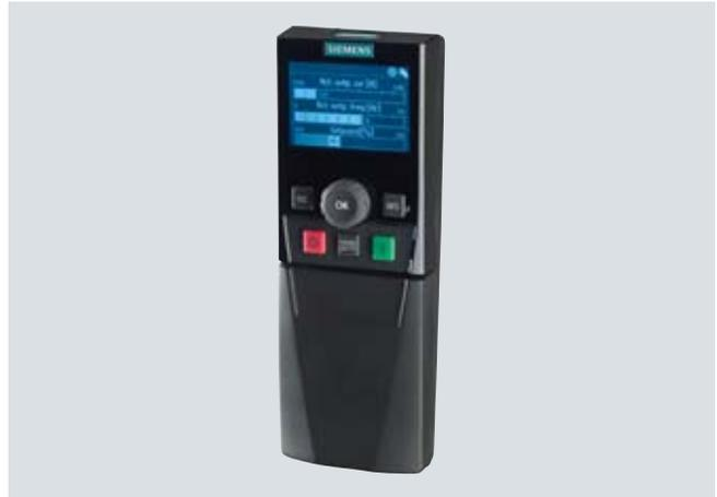
A handheld version of the IOP can be ordered for mobile use. In addition to the IOP, this includes a housing with rechargeable batteries, charging unit and RS232 interface cable. The charging unit is supplied with connector adapters for Europe, the US and UK. When the batteries are fully charged, the operating time is up to 8 hours.
