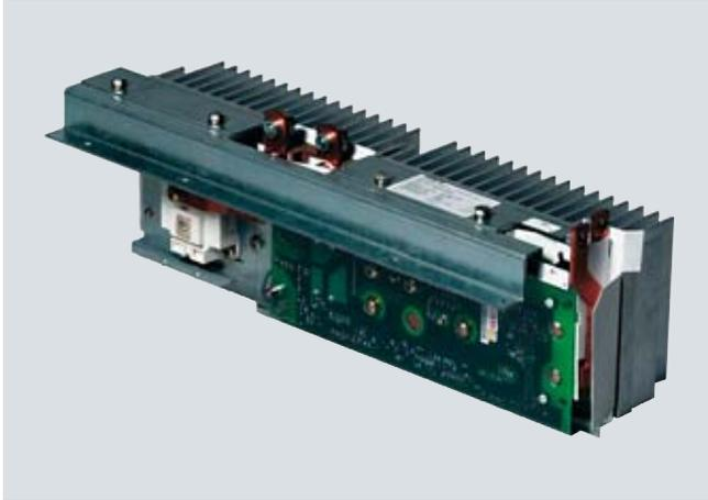
A Braking Module and the matching external braking resistor are required to bring drives to a controlled standstill in the event of a power failure (e.g. emergency retraction or EMERGENCY STOP Category 1) or limit the DC link voltage for brief periods of generator operation. The Braking Module includes the power electronics and the associated control circuit. During operation, the DC link energy is converted to heat loss in an external braking resistor. Braking Modules function autonomously.
