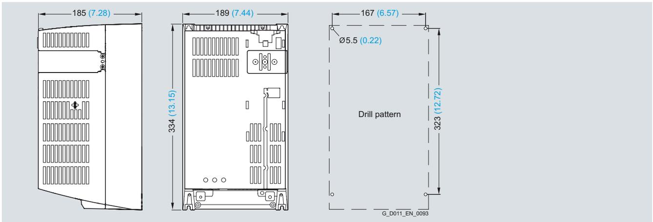
PM250 Power Module frame size FSC with integrated class A line filter
