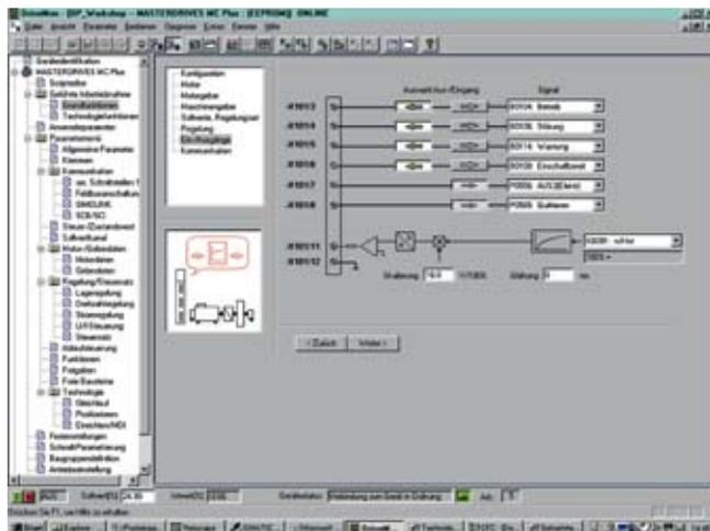
Drive ES is the engineering system used to integrate the communication, configuration and data management functions of Siemens drive technology into the SIMATIC automation world easily, efficiently and cost-effectively. The STEP 7 Manager user interface provides the ideal basis for this.
