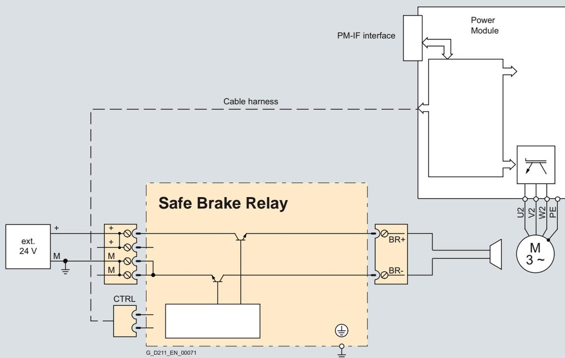
Connection example of a Safe Brake Relay
