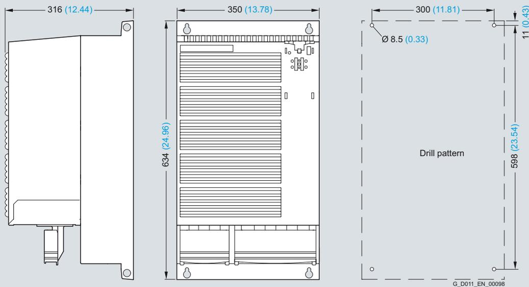
PM260 Power Module frame size FSF with and without integrated line filter class A
