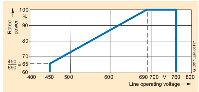
The power units can be operated with 500 V –10 %. In this case, the power is reduced linearly as required.
