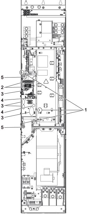
Figure 11-12 Replacing the Control Interface Module, Power Module, frame size  $\mathsf{GX}$
