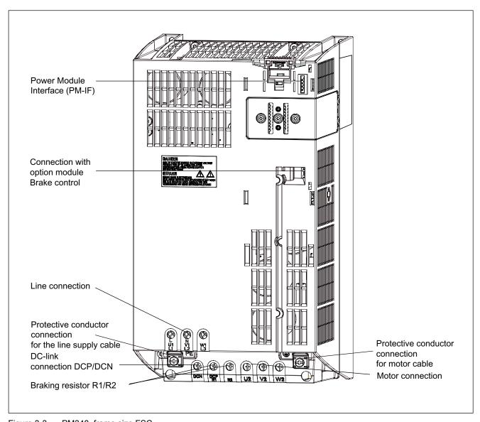
Figure 3-3 PM340, frame size FSC
