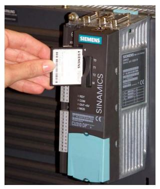
Figure 6-4 Slot for CompactFlash card
