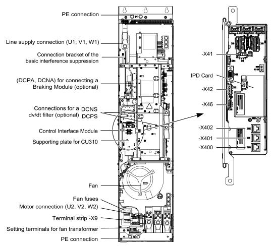
Figure 3-50 Power Module, frame size FX, with order number 6SL3310-1TE32-xAA3
