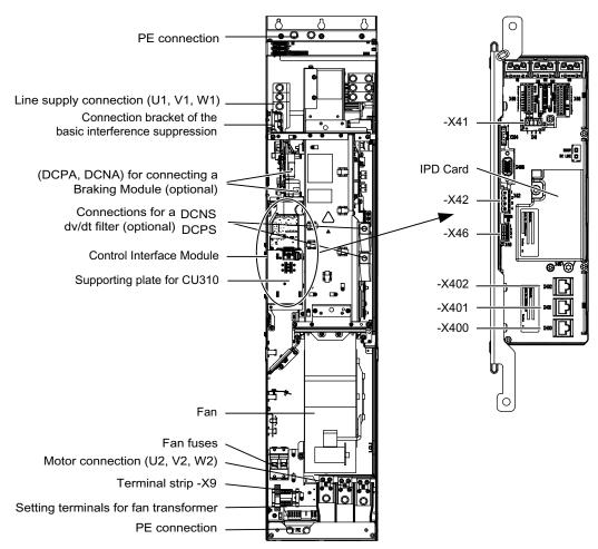
Figure 3-52 Power Module, frame size GX, with order number 6SL3310-1TE3x-xAA3
