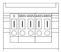
Figure 3-59 Setting terminals for the fan transformers
