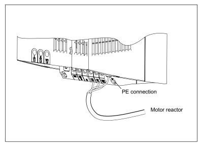
Figure 5-10 Electrical connection
