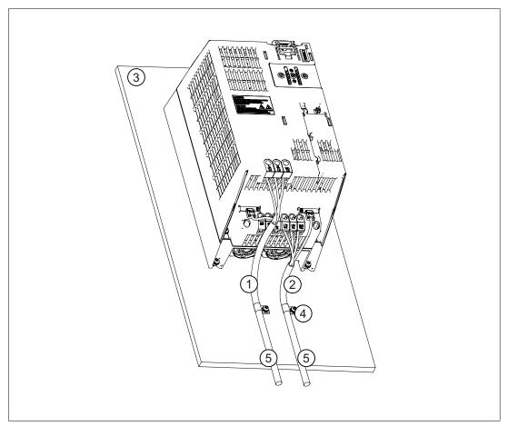
Figure 9-2 Shielding of a Power Module PM340
