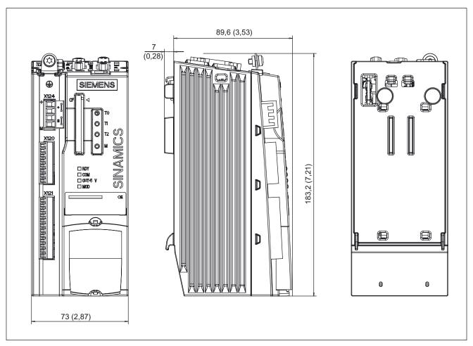
Figure 6-9 Dimension drawing, CU310 PN
