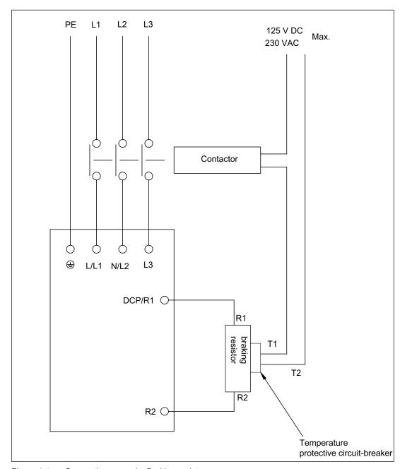
Figure 4-1 Connection example: Braking resistor
