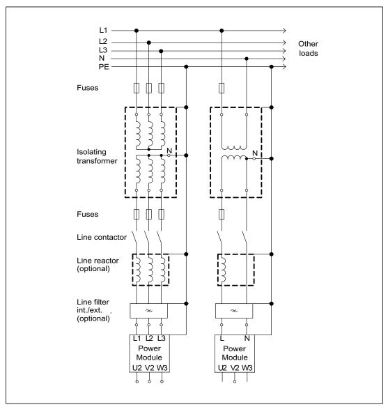
Figure 2-6 Isolating transformer
