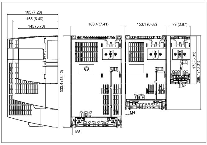
Figure 3-9 Dimension drawings, Power Module PM340
