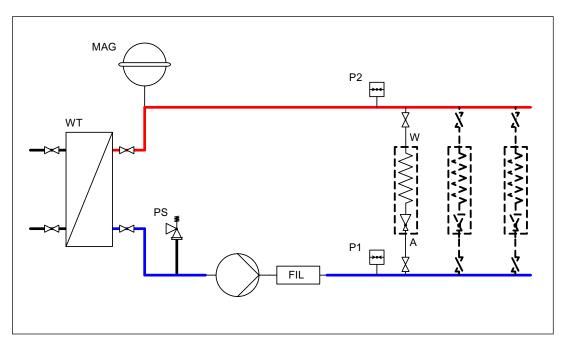
Figure 10-1 Example: Closed cooling circuit
