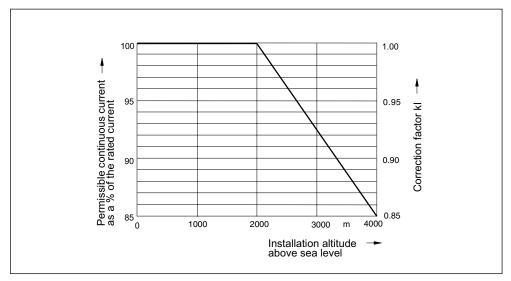
Figure 3-63 Current correction factor as a function of installation altitude
