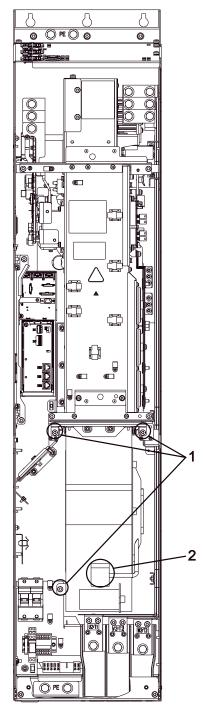
Figure 11-15 Replacing the fan, Power Module, frame size  $\mathsf{GX}$
