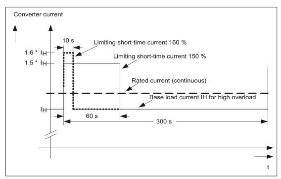
Figure 3-61 High overload
