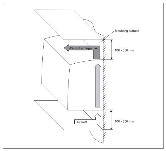
Figure 9-3 Cooling clearances
