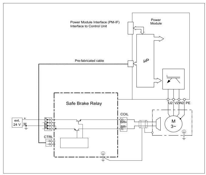
Figure 7-13 Connection example: Safe Brake Relay
