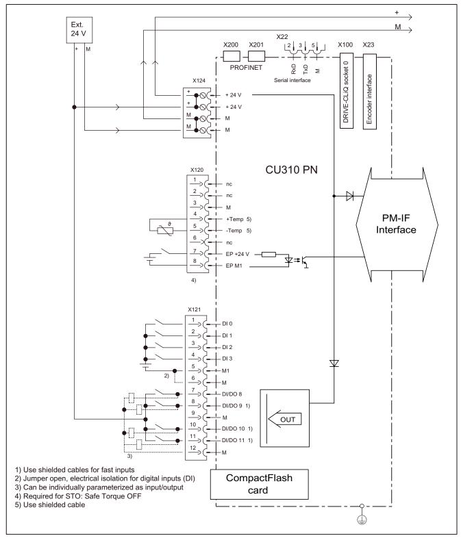
Figure 6-8 Connection example CU310 PN
