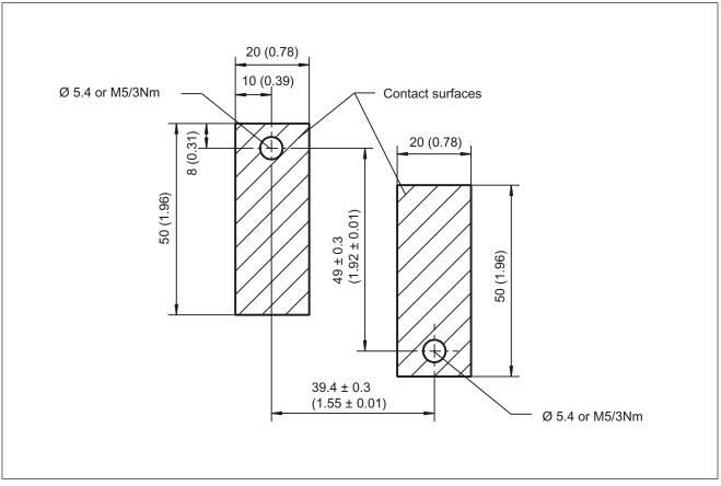
Figure 8-7 Hole drilling template for installation
