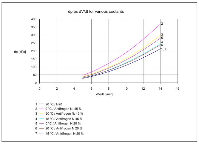
Figure 10-4 Pressure difference as a function of the volumetric flow for Power Modules PM340 Liquid Cooled, frame sizes FSD to FSF
