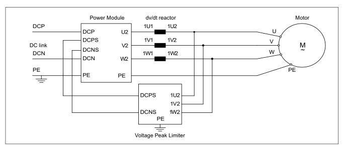
Figure 5-15 Connecting the dv/dt filter plus Voltage Peak Limiter
