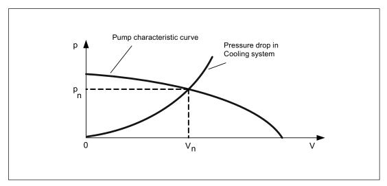
Figure 10-2 Pump characteristic curve
