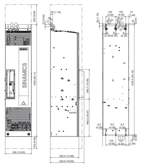
Figure 3-56 Dimension drawing Power Module, frame size FX
