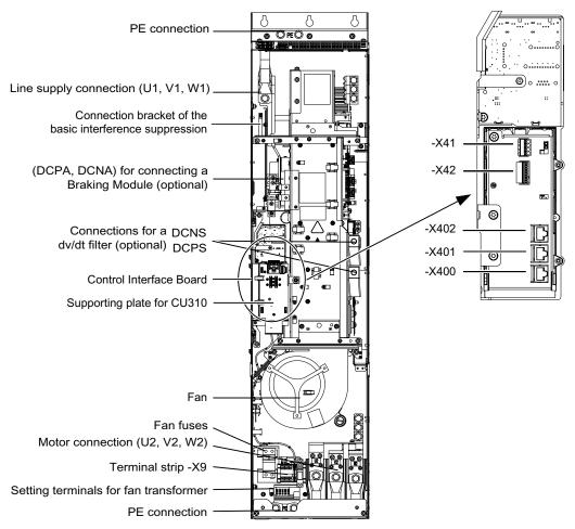
Figure 3-51 Power Module, frame size FX, with order number 6SL3310-1TE32-xAA0
