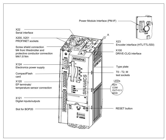
Figure 6-7 Description of the CU310 PN interfaces
