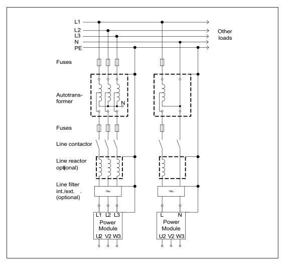
Figure 2-5 Autotransformer
