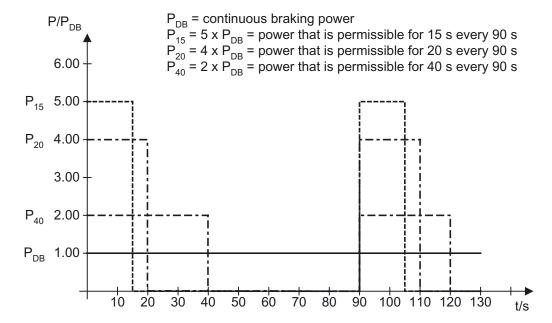
Figure 4-14 Duty cycle for braking resistors
