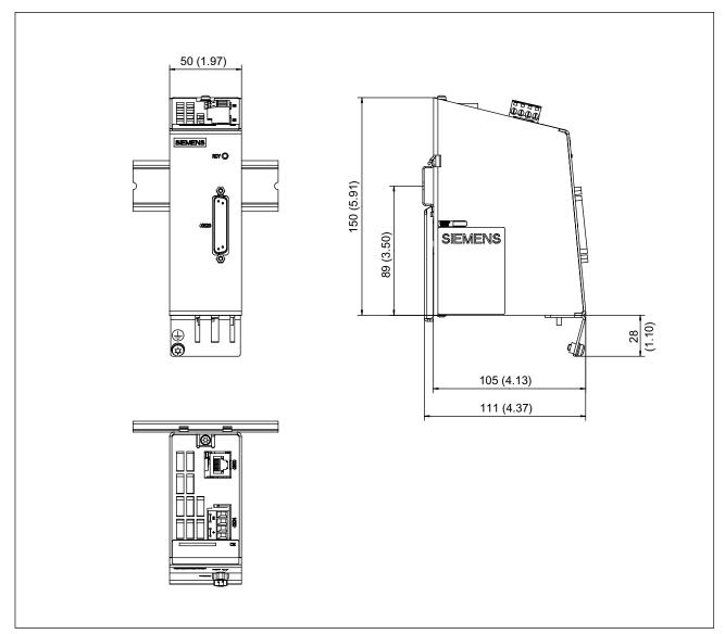
Figure 7-4 Dimension drawing of the SMC10
