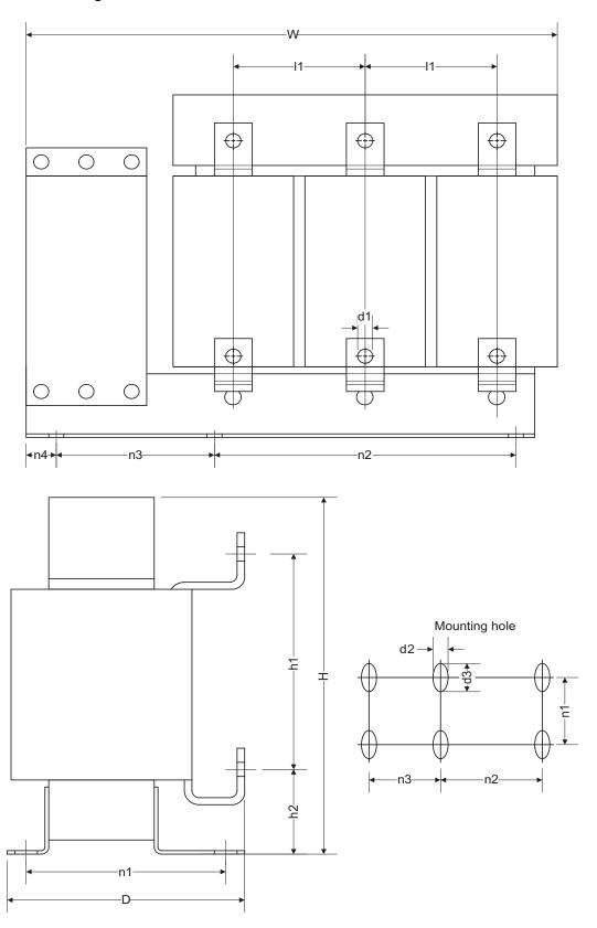
Figure 5-12 Dimension drawing, sinusoidal filter
