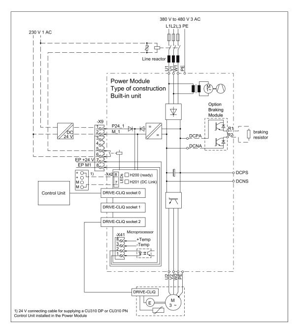
Figure 3-55 Connection example: Power Module built-in unit with order number 6SL3310-1TE3x-xAA0
