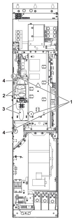
Figure 11-13 Replacing the Control Interface Board, Power Module, frame size GX
