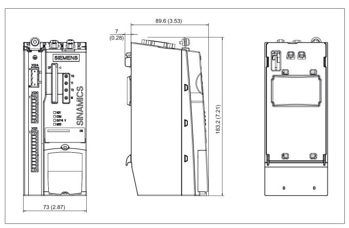
Figure 6-5 Dimension drawing CU310 DP
