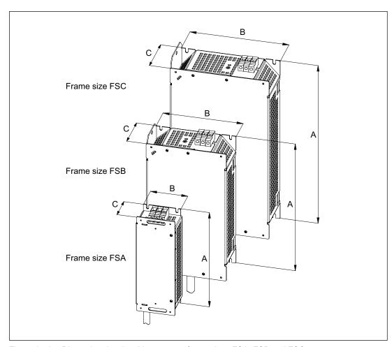
Figure 2-10 Dimension drawing: Line reactor, frame sizes FSA, FSB and FSC
