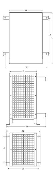
Figure 4-3 Dimension drawing: Braking resistor, frame sizes FSC, FSD, FSE, FSF
