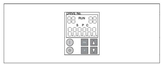
Figure 7-2 Overview of displays and keys
