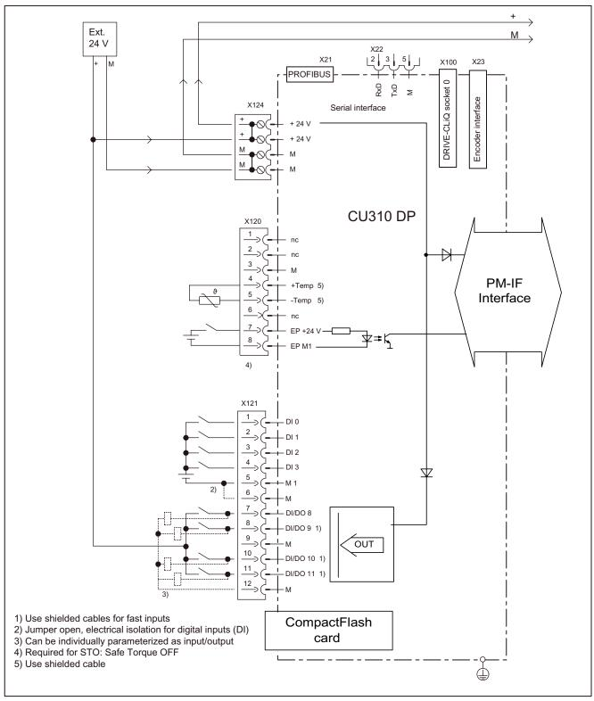
Figure 6-3 Connection example CU310 DP
