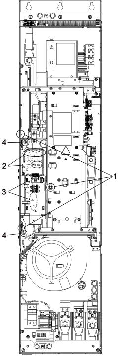
Figure 11-11 Replacing the Control Interface Board, Power Module, frame size FX
