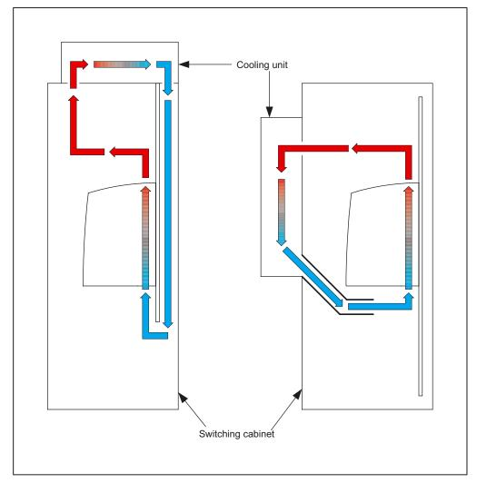
Figure 9-4 Examples of cabinet ventilation
