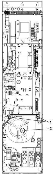
Figure 11-14 Replacing the fan, Power Module, frame size FX
