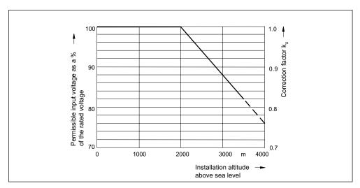
Figure 3-64 Voltage correction factor as a function of installation altitude
