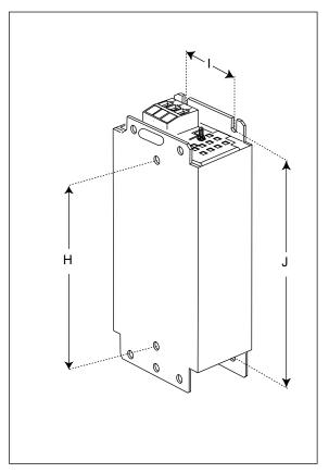
Figure 2-14 Mounting: Line reactor, frame size FSA
