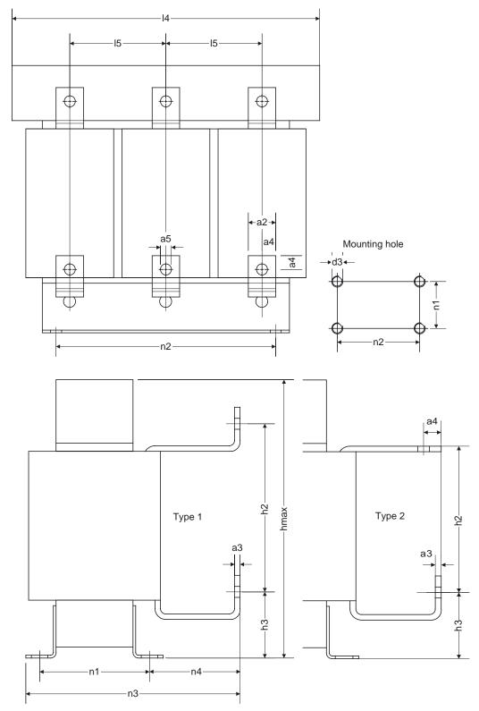
Figure 5-11 Dimension drawing, motor reactor
