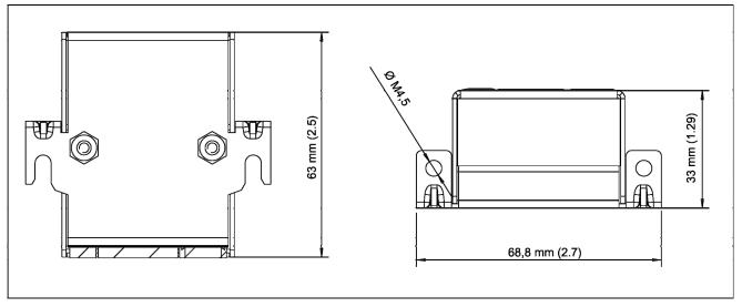
Figure 7-14 Dimension drawing: Safe Brake Relay
