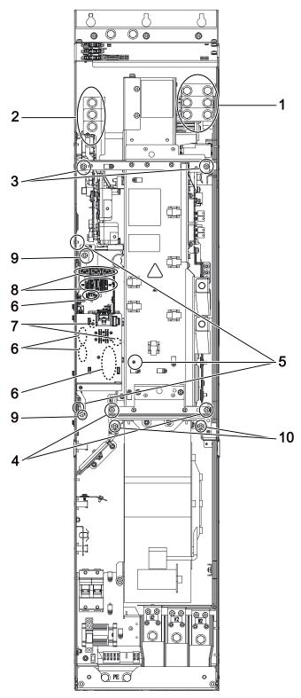
Figure 11-9 Replacing the Powerblock, Power Module, frame size GX
