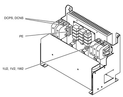
Figure 5-14 Interface overview, voltage peak limiter, type 2
