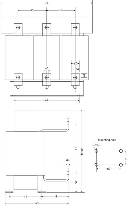
Figure 2-13 Dimension drawing, line reactors
