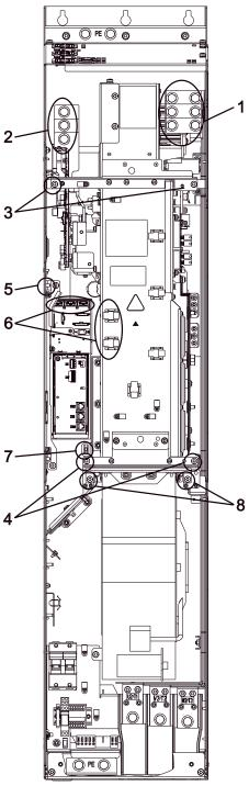
Figure 11-8 Replacing the Powerblock, Power Module, frame size GX
