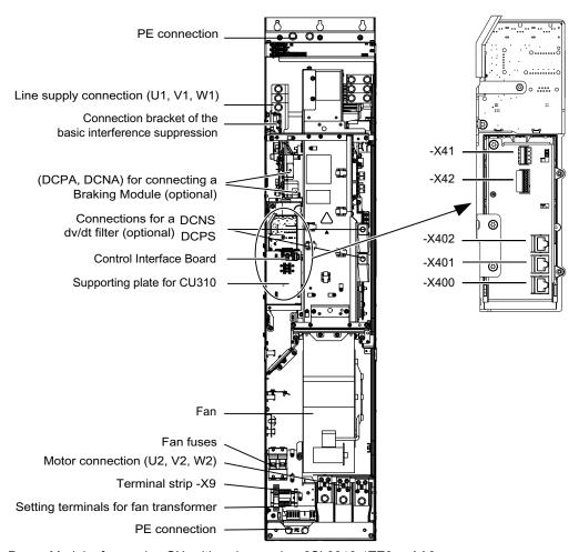
Figure 3-53 Power Module, frame size GX, with order number 6SL3310-1TE3x-xAA0
