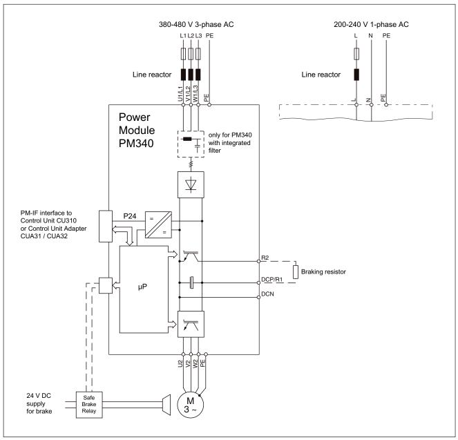
Figure 3-7 PM340 connection example
