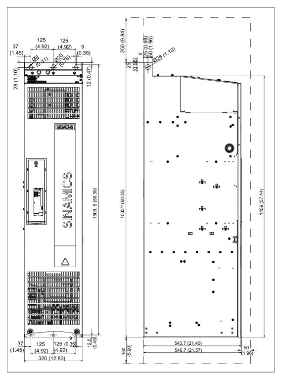
Figure 3-57 Dimension drawing Power Module, frame size GX
