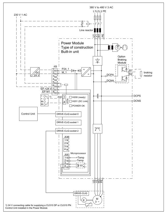
Figure 3-54 Connection example: Power Module built-in unit with order number 6SL3310-1TE3x-xAA3
