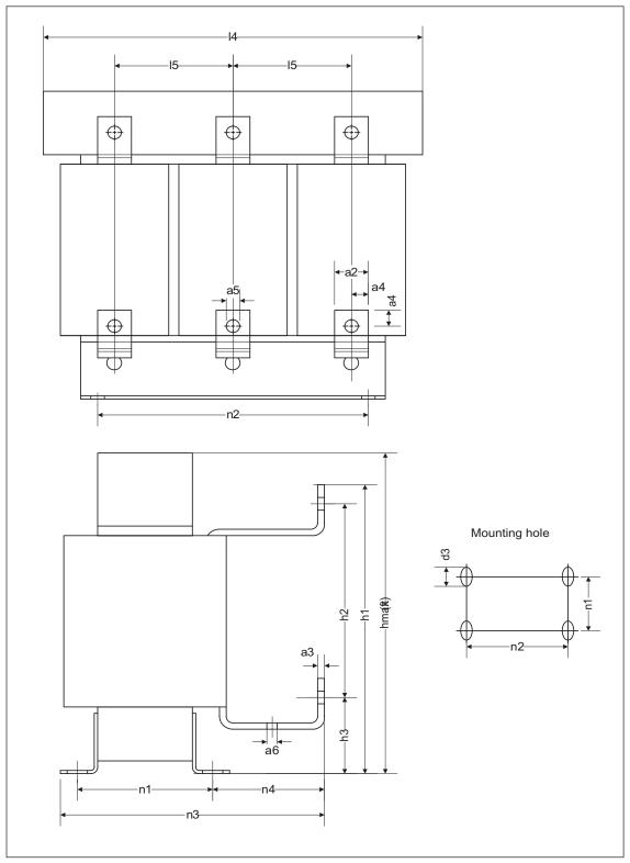
Figure 5-16 Dimension drawing, dv/dt reactor
