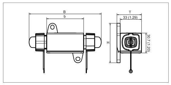
Figure 8-6 Dimension drawing, DRIVE-CLiQ coupling
