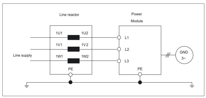
Figure 2-18 Power Module with line filter
