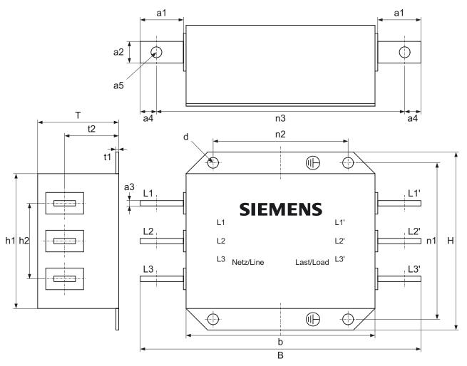
Figure 2-8 Dimension drawing, line filter
