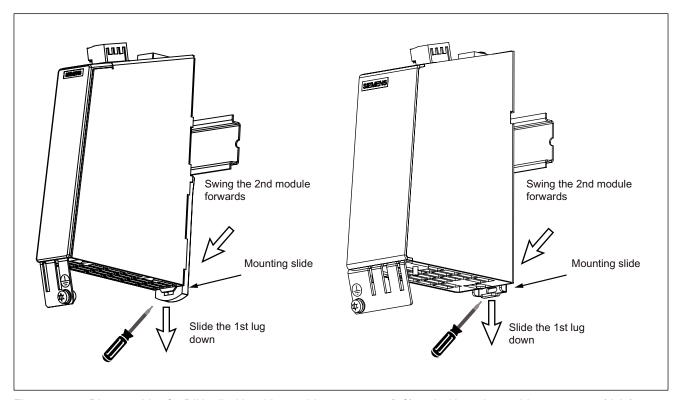
Figure 7-11 Disassembly of a DIN rail with a 30mm wide component (left) and with a 50mm wide component (right).
