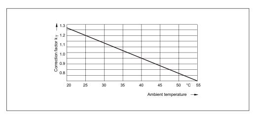
Figure 3-62 Current correction factor as a function of ambient temperature
