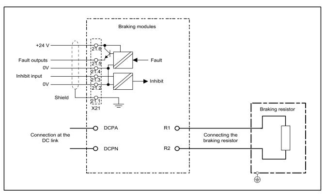
Figure 4-7 Example connection of Braking Module
