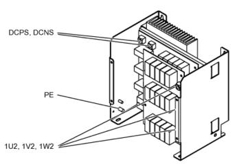
Figure 5-13 Interface overview, voltage peak limiter, type 1
