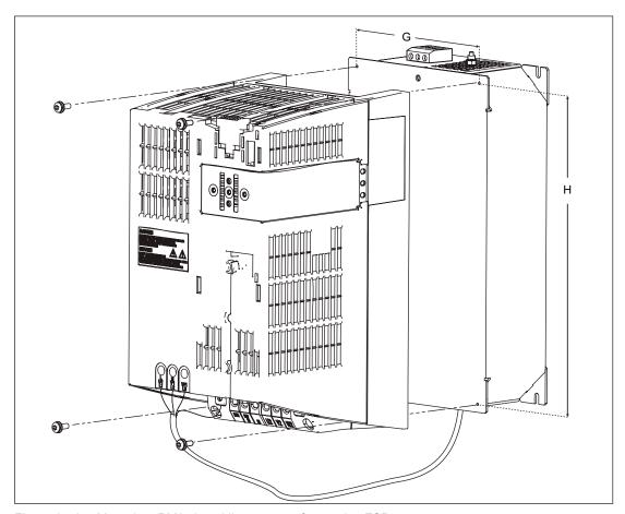
Figure 2-16 Mounting: PM340 and line reactor, frame size FSB
