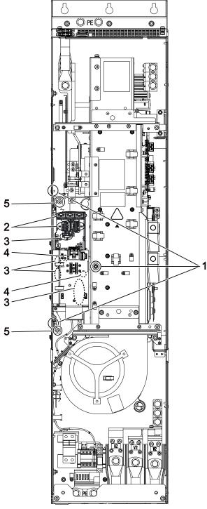
Figure 11-10 Replacing the Control Interface Module, Power Module, frame size FX
