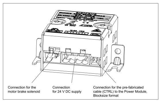
Figure 7-12 Interface description: Safe Brake Relay
