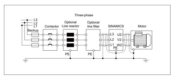
Figure 2-1 Example of a blocksize line connection
