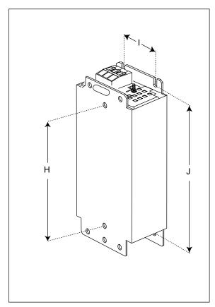
Figure 2-11 Mounting: Line reactor, frame size FSA
