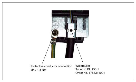
Figure 7-20 Shield contacts for the SMC30
