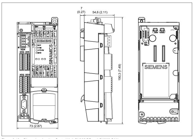
Figure 6-10 Dimension drawing: Control Unit CU305 DP and CU305 CAN
