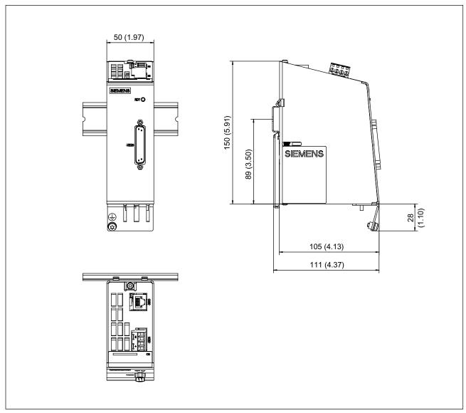
Figure 7-4 Dimension drawing of the SMC10
