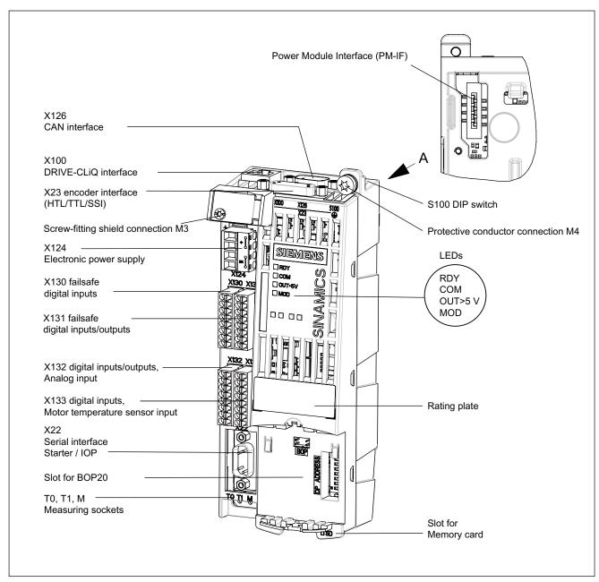
Figure 6-2 Interface description CU305 CAN
