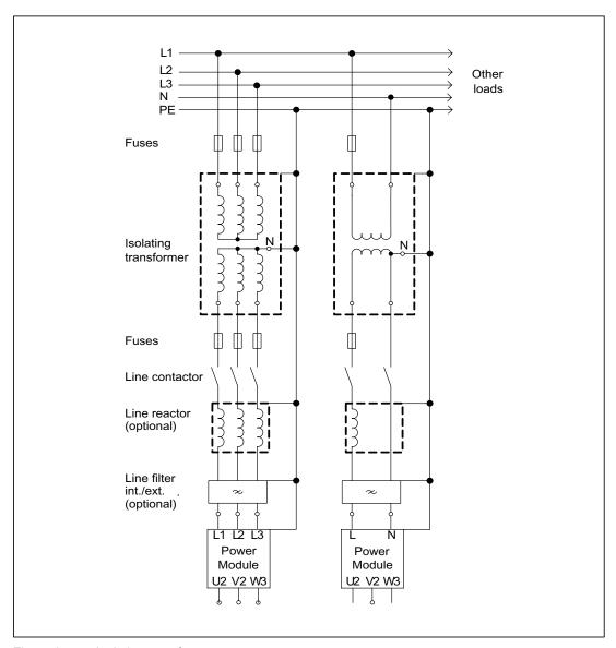
Figure 2-5 Isolating transformer
