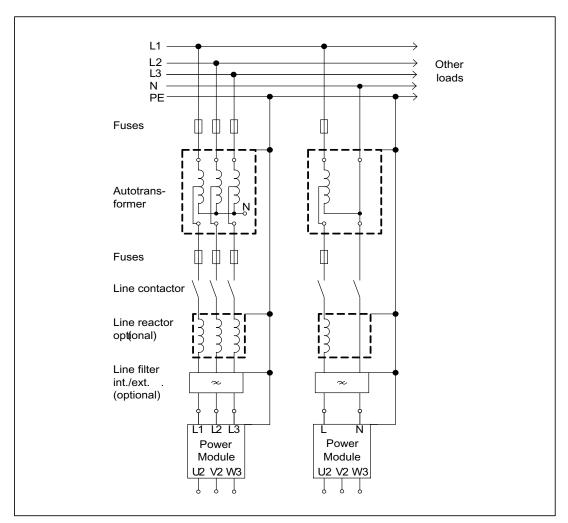
Figure 2-4 Autotransformer
