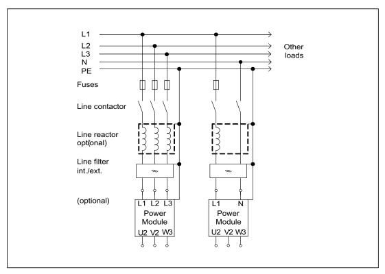
Figure 2-3 Direct operation on the line supply
