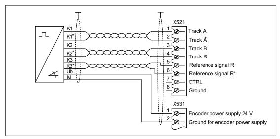
Figure 7-14 Connection example 1: HTL encoder, bipolar, with reference signal
