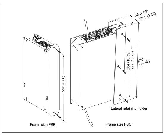
Figure 2-14 Side mounting: Line reactors, frame sizes FSB and FSC
