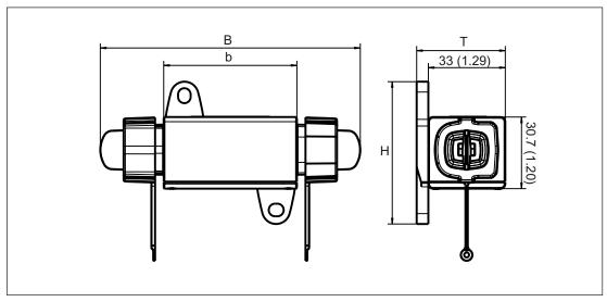
Figure 8-6 Dimension drawing, DRIVE-CLiQ coupling
