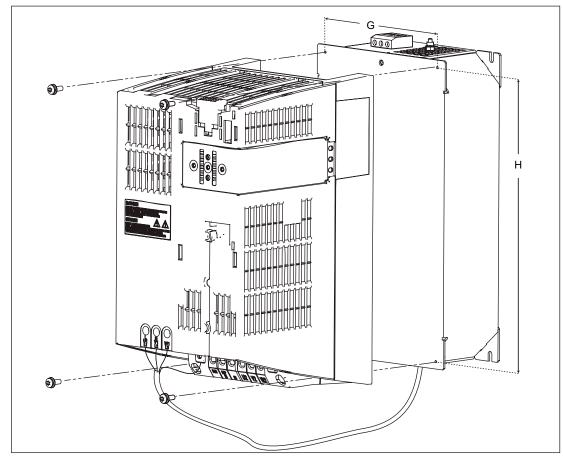
Figure 2-13 Mounting: PM340 and line reactor, frame size FSB
