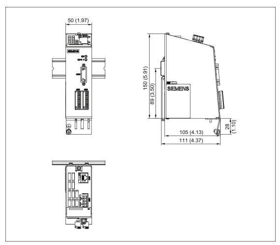
Figure 7-17 Dimension drawing SMC30: 50 mm wide
