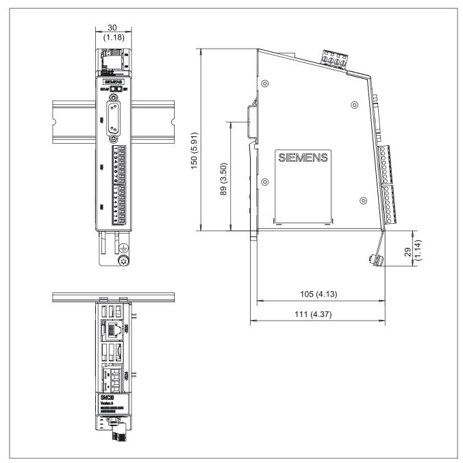
Figure 7-16 Dimension drawing SMC30: 30 mm wide
