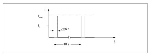
Figure 3-20 Load cycle without pre-load condition (for servo drives)
