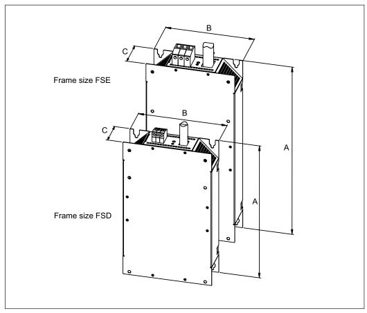
Figure 2-9 Dimension drawing: Line reactor, frame sizes FSD and FSE
