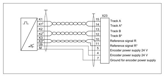
Figure 6-7 Connection example 1: HTL encoder, bipolar, with reference signal
