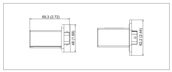
Figure 8-2 Dimensions of the DRIVE-CLiQ cabinet gland, all dimensions in mm and (inches)
