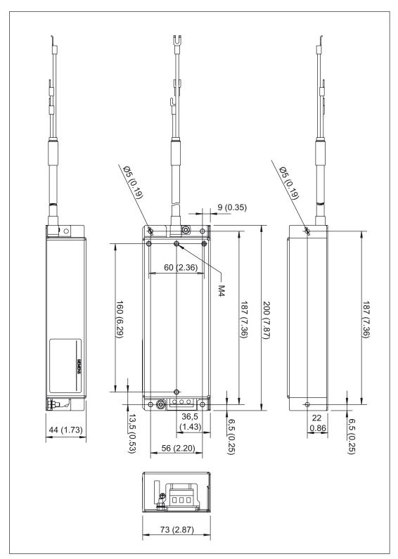
Figure 2-6 Dimension drawing: Line filter, frame size FSA
