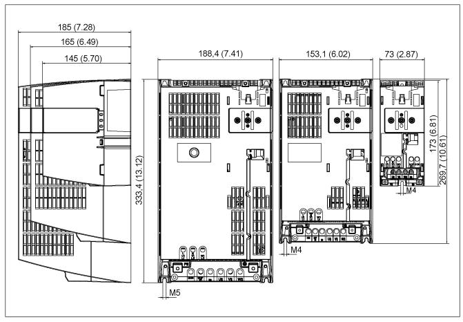
Figure 3-9 Dimension drawings, Power Module PM340
