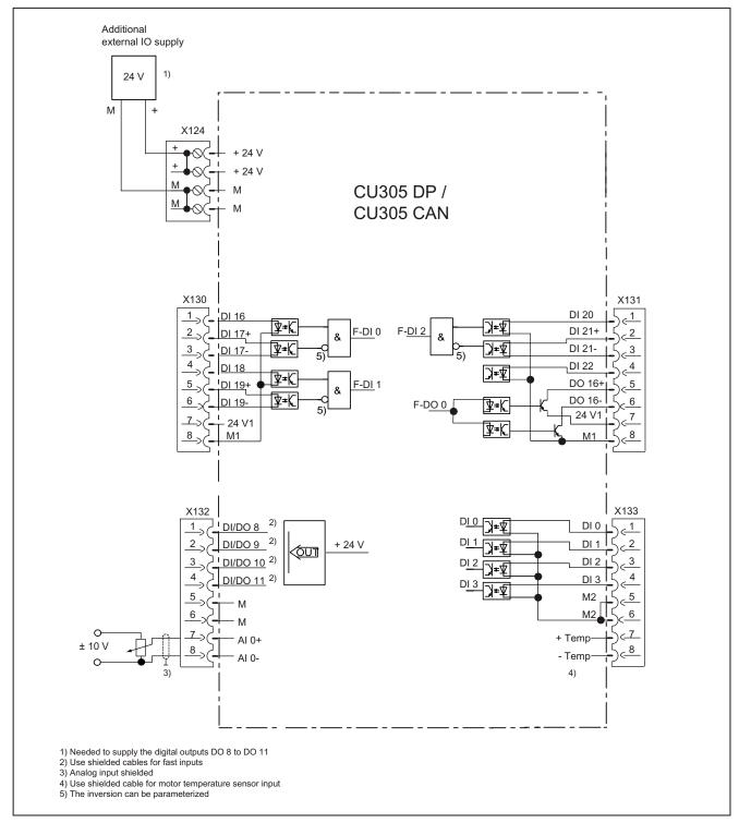
Figure 6-5 Internal connections of the CU305 with the safety function
