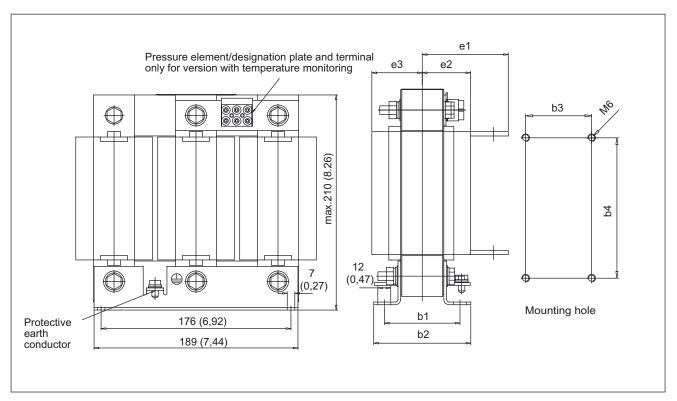
Figure 5-3 Dimension drawing: Motor reactor, frame size FSD
