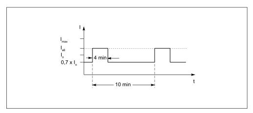
Figure 3-21 S6 load cycle with pre-load condition (for servo drives)
