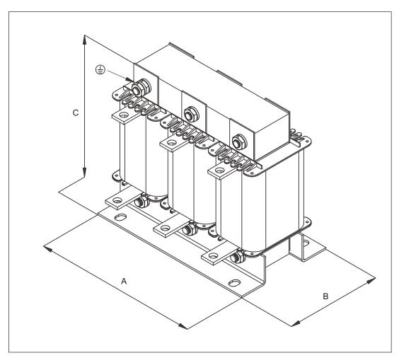
Figure 2-10 Dimension drawing: Line reactor, frame size FSF
