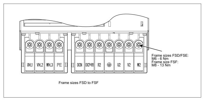
Figure 3-32 Arrangement of the line supply and motor terminals for the PM340
