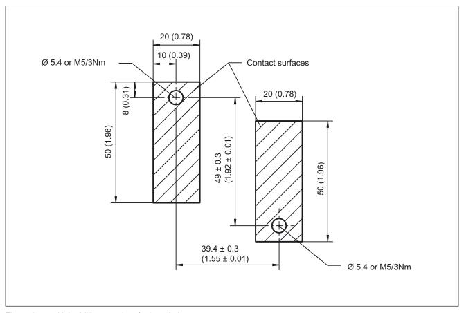
Figure 8-7 Hole drilling template for installation
