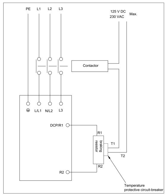
Figure 4-1 Connection example: Braking resistor
