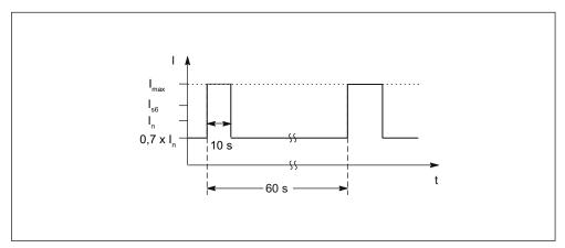
Figure 3-22 Load cycle with pre-load condition (for servo drives)
