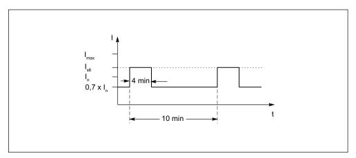
Figure 3-41 S6 load cycle with pre-load condition (for servo drives)
