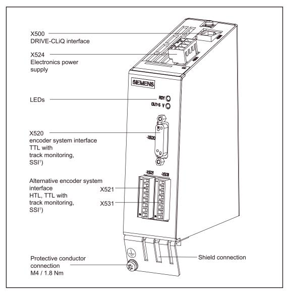
Figure 7-13 Interface description SMC30, 50 mm wide, order no. 6SL3055-0AA00-5CA0, 6SL3055-0AA00-5CA1
