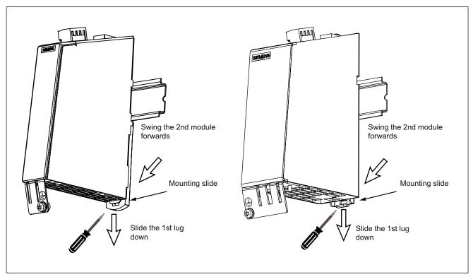
Figure 7-11 Disassembly of a DIN rail with a 30mm wide component (left) and with a 50mm wide component (right).
