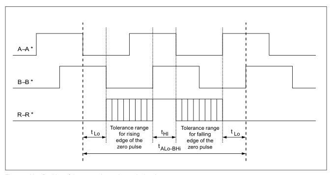
Figure 7-23 Position of the zero pulse to the track signals
