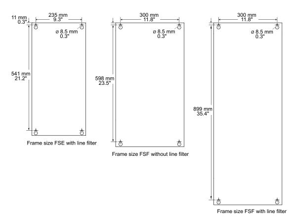
Figure 3-17 Drilling templates for frame sizes FSD to FSF - with and without line filter
