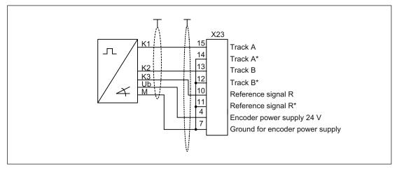
Figure 6-8 Connection example 2: HTL encoder, unipolar, with reference signal 1)
