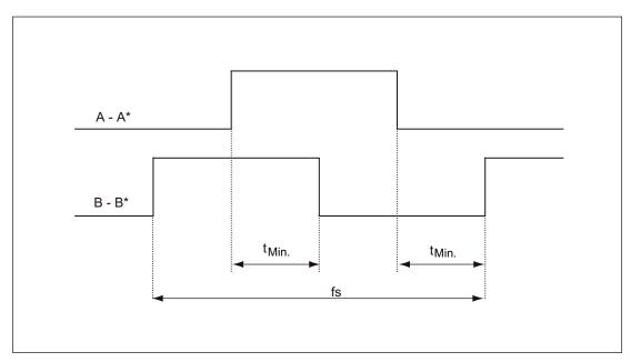
Figure 7-22 Signal characteristic of track A and track B between two edges: Time between two edges with pulse encoders
