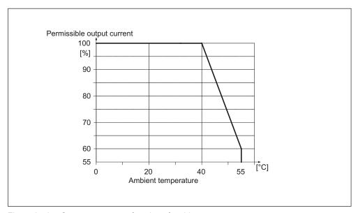
Figure 3-46 Output power as a function of ambient temperature
