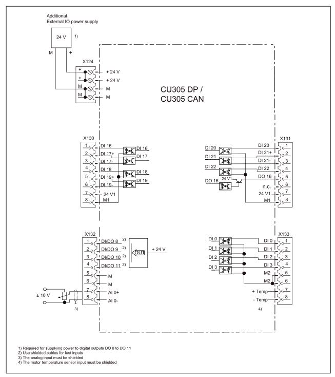
Figure 6-3 Internal connections of the CU305 without the safety function
