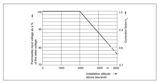
Figure 3-28 Voltage correction factor as a function of installation altitude
