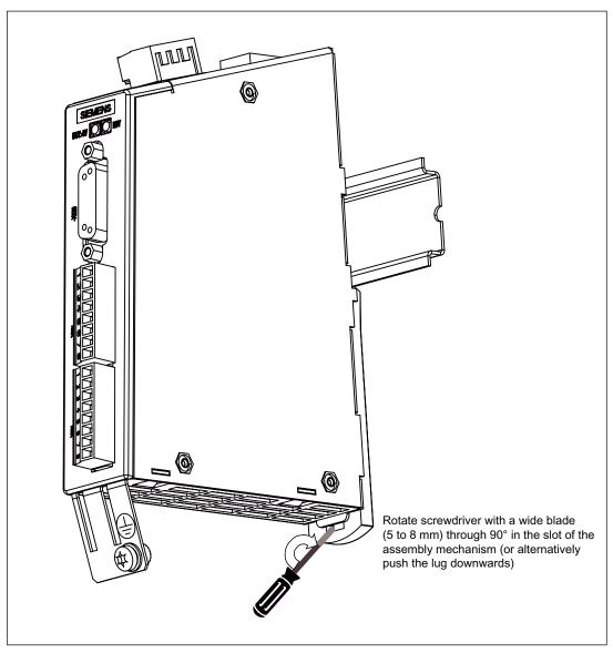
Figure 7-19 Removing: SMC30: 30 mm wide
