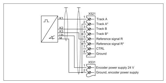
Figure 7-15 Connection example 2: HTL encoder, unipolar, with reference signal<sup>1)</sup>
