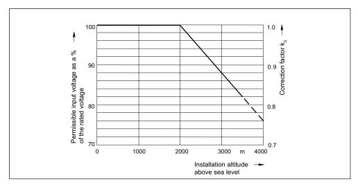
Figure 3-48 Voltage correction factor as a function of installation altitude
