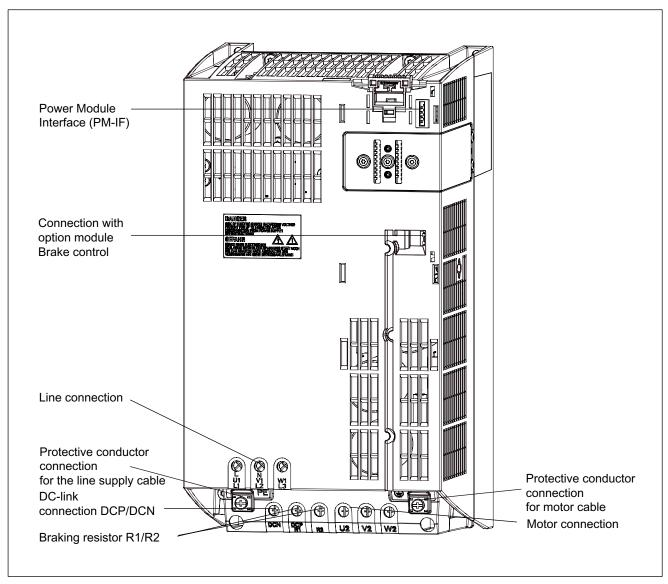
Figure 3-3 PM340, frame size FSC
