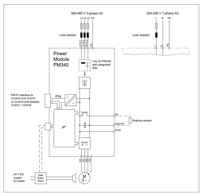
Figure 3-7 PM340 connection example
