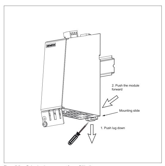
Figure 7-5 Releasing the component from a DIN rail
