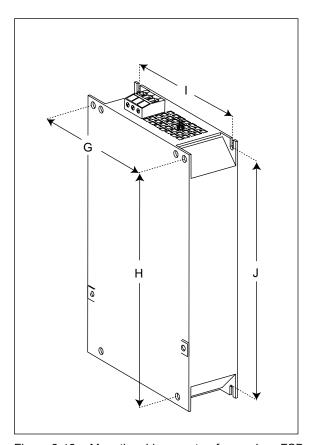
Figure 2-12 Mounting: Line reactor, frame sizes FSB and FSC
