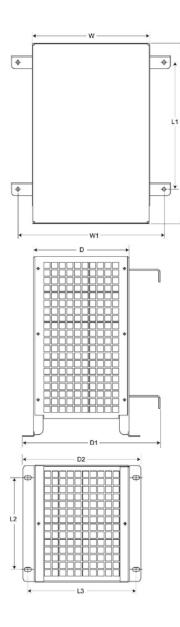
Figure 4-3 Dimension drawing: Braking resistor, frame sizes FSC, FSD, FSE, FSF
