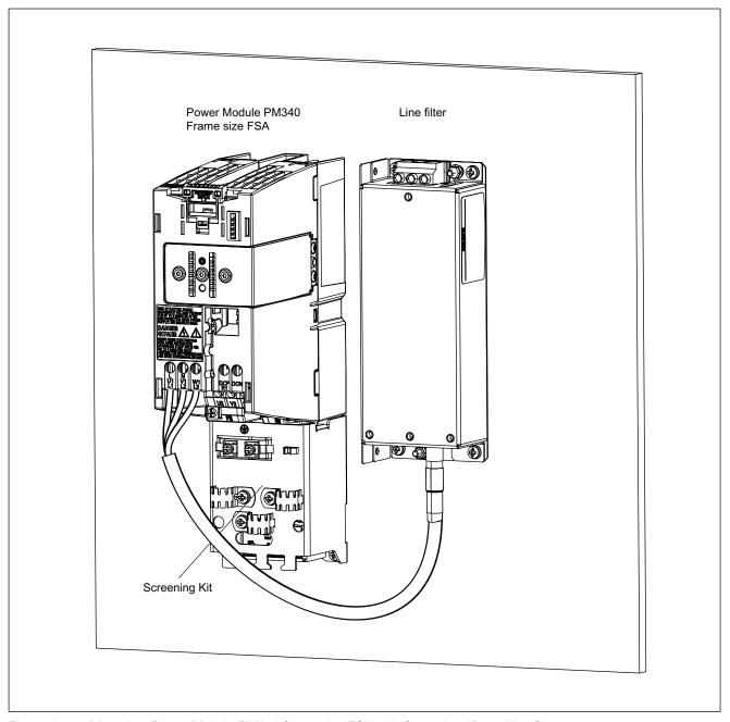
Figure 2-7 Mounting: Power Module PM340 frame size FSA with Screening Kit and line filter
