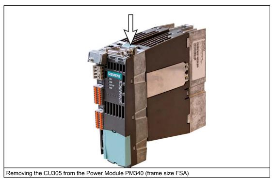
In order to remove the Control Unit from the Power Module, the blue release lever, as shown in the diagram, must be pressed downwards and the Control Unit swung out to the front.
