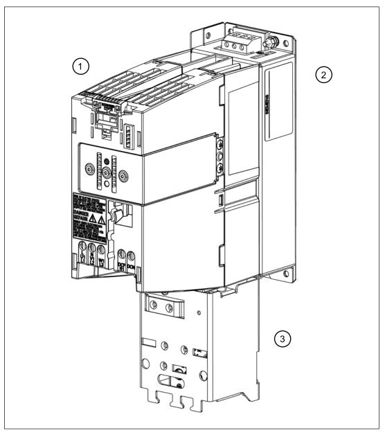
Figure 8-19 Power Module PM340, frame size FSA, with line filter and Screening Kit
