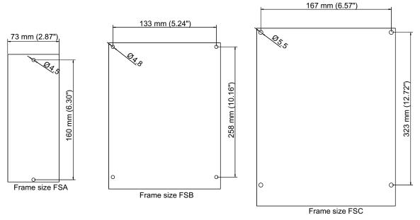
Figure 3-16 Drilling templates for frame sizes FSA and FSC
