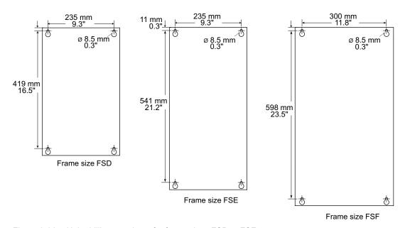
Figure 3-36 Hole drilling templates for frame sizes FSD to FSF
