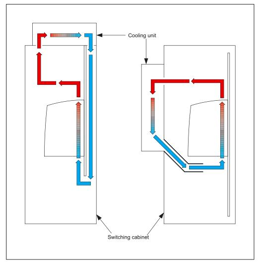
Figure 9-4 Examples of cabinet ventilation
