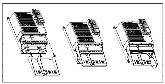
Figure 8-20 Mounting: Power Module PM340 liquid cooled, frame size FSD and Screening Kit
