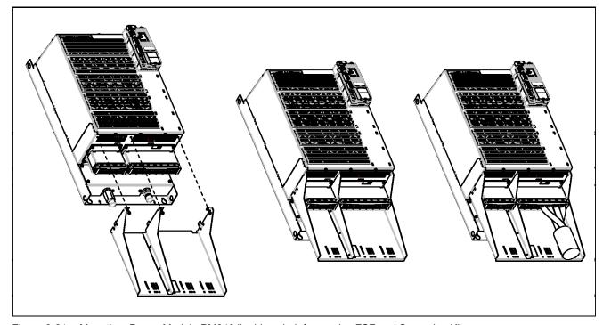
Figure 8-21 Mounting: Power Module PM340 liquid cooled, frame size FSF and Screening Kit
