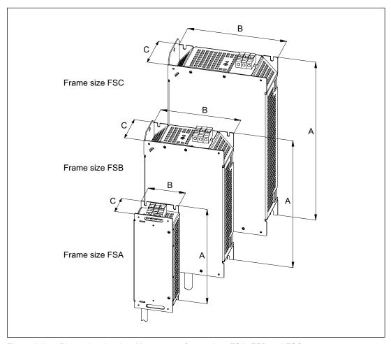
Figure 2-8 Dimension drawing: Line reactor, frame sizes FSA, FSB and FSC
