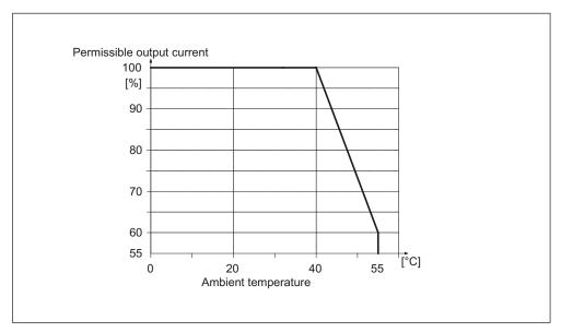
Figure 3-26 Output power as a function of ambient temperature
