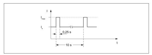
Figure 3-39 Load cycle with pre-load condition (for servo drives)
