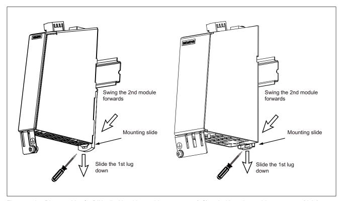
Figure 7-18 Disassembly of a DIN rail with a 30mm wide component (left) and with a 50mm wide component (right).
