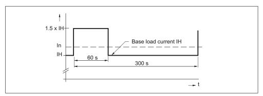
Figure 3-43 Load cycle with 60 s overload with a load cycle period of 300 s
