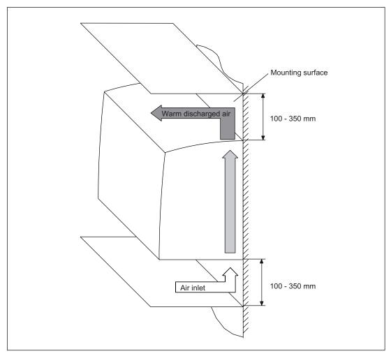
Figure 9-3 Cooling clearances
