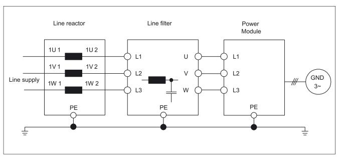
Figure 2-16 Power Module Blocksize with line reactor and line filter
