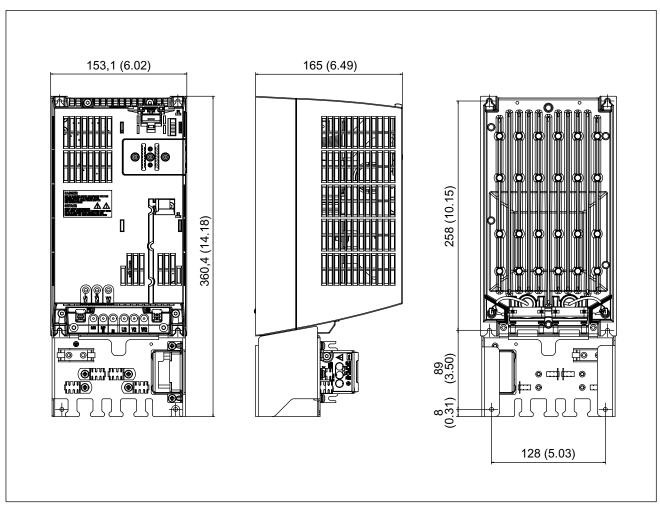
Figure 8-10 Dimension drawing: Power Module PM340 with Screening Kit and Brake Relay, frame size FSB
