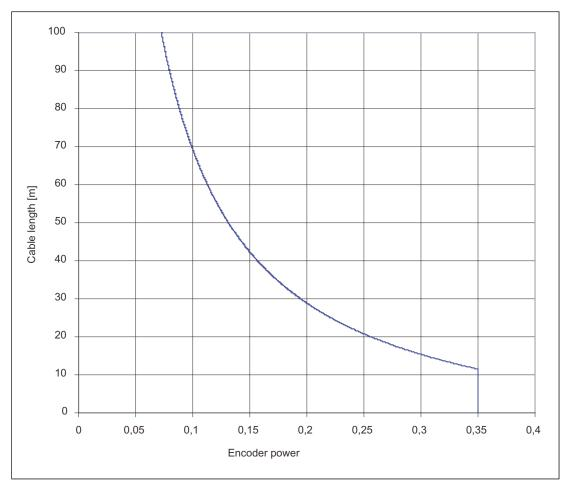
Figure 7-21 Max. cable length as a function of the encoder current drawn
