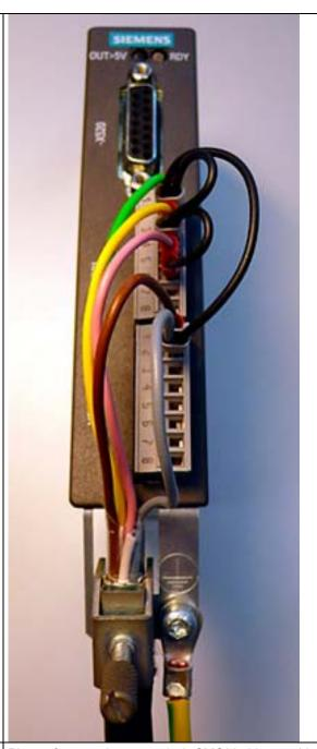
Photo of connection example 2: SMC30, 30 mm wide, from Order No. 6SL3055-0AA00-5CA2 and Firmware 2.5 SP1
