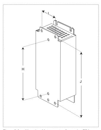
Figure 5-6 Mounting: Motor reactor, frame size FSA
