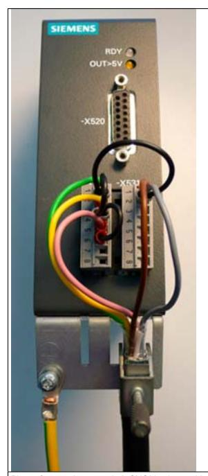
Photo of connection example 2: SMC30, 50 mm wide (Order No. 6SL3055-0AA00-5CA0, 6SL3055-0AA00-5CA1)
