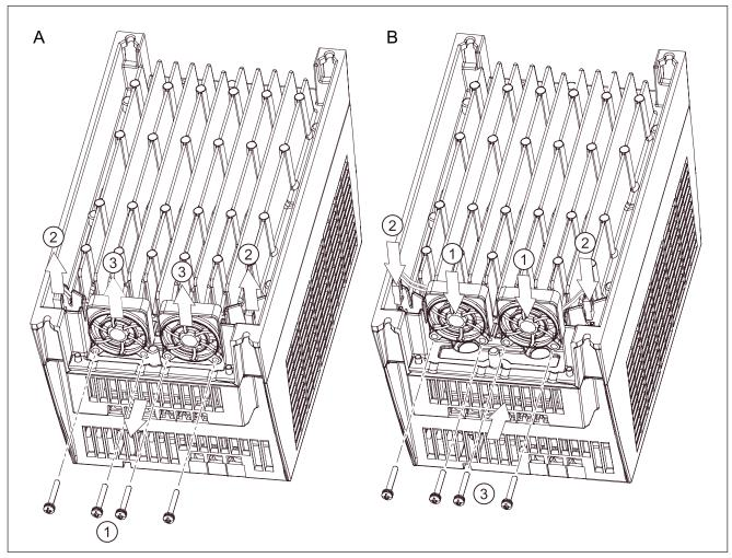
Figure 10-2 Replacing a fan for a Power Module PM340, frame sizes FSB and FSC
