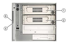
Figure 7-4 Drives in the exchangeable rack
