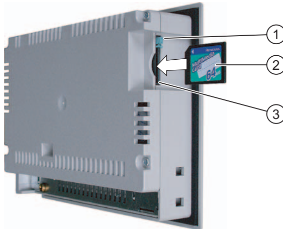
Figure 5-3 Inserting a memory card – TP 177B as an example
