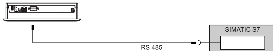
Figure 4-9 Connecting a controller to a TP 177A
